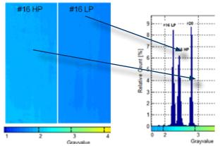
The Histogram can differentiate between materials of the same thickness, but with different porosities
