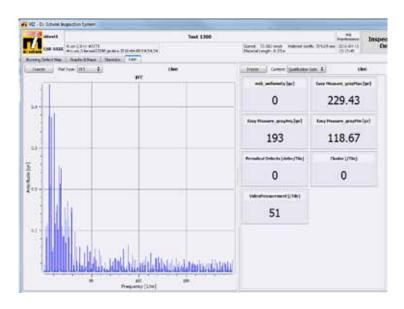
The uniformity in fiber distribution has a strong influence on the nonwoven web performance. This includes more cosmetic properties such as cloudiness, but also functional properties such as web thickness specifying the stability of a nonwoven material.
