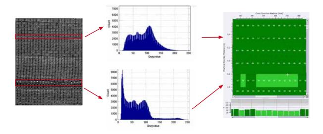
Histogram distribution for good material (top) and misaligned meshes (bottom). The histogram values are then applied to the tiles, and show where the material is outside the specification.
