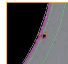
Glass Edge Defect at Drill Hole
